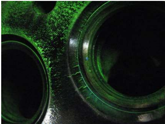
Figure 2. Cracks in the valve seat produced by thermal stress.
