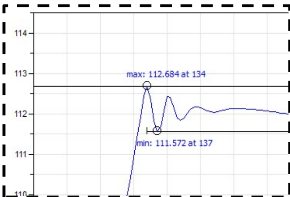
Figure 16. Dymola initial Thermalshock 2 stability estimated as \pm 0.6^{\circ}\text{C} with only low frequency and amplitude oscillations.
